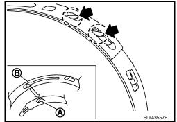
ii. Pinch projection on the band with suitable pliers to tighten band.
