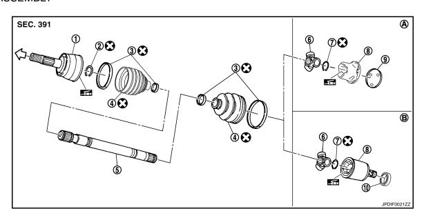
1. Joint sub-assembly 2. Circular clip 3. Boot band
