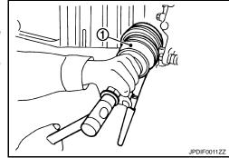
25. Install the boot securely into grooves (indicated by "\*" marks) shown in the figure.
