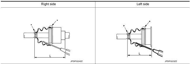
11. To prevent the deformation of the boot, adjust the boot installation length (L) to the value shown below by inserting the suitable tool into the inside of boot from the large diameter side of boot and discharging inside air.
